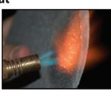
Actual disk of HeatShield Cerfractory heated with torch
