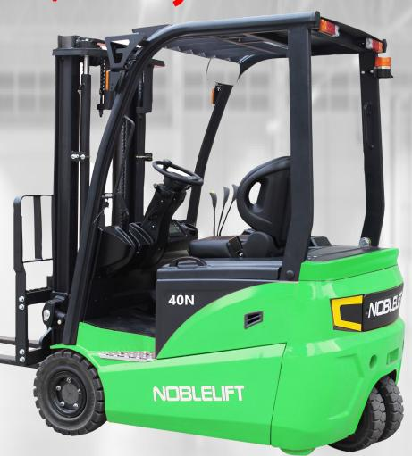
\* 3500-4000lbs. Lift Capacity \* 189" Lift Height \* 42" Forks \* Side Shifting / Fork Positioner \* 48V/400Ah Lithium Iron Phosphate Battery \* 48V/200Ah 3 Phase Charger \* Warning Beacon \* F/R Work Lights \* Rear Blue Light \* 3-Way Valve \* Rear Grab Bar w/ Horn \* Comfort Seat \* Solid Pneumatic Tires
