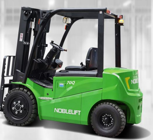
\* 5000-7000lbs Lift Capacity \* 189" Lift Height \* 42" Forks \* Side Shifting / Fork Positioner \* 80V/400Ah Lithium Iron Phosphate Battery \* 80V/200Ah 3 Phase Charger \* Warning Beacon \* F/R Work Lights \* Rear Blue Light \* 3-Way Valve \* Rear Grab Bar w/ Horn \* Comfort Seat \* Solid Pneumatic Tires
